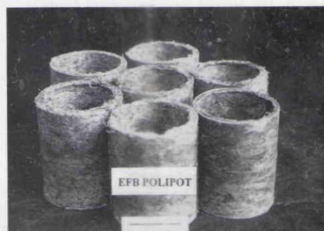
Figure 6. EFB-Polipot made from empty fruit bunch fiber
